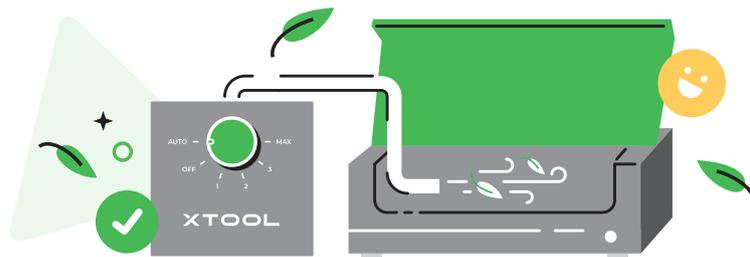
An air assist set draws in air and blows it into a laser machine through an air tube. The airflow can be adjusted. Generally, a small airflow is used to clean the processing area and cool the processed material part during laser engraving, and a large airflow is used in laser cutting not only for cleaning and cooling but also for smoke exhaustion and residue blowing.
