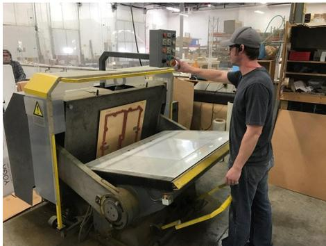
A die is created that presses into the cut material, making the part.
