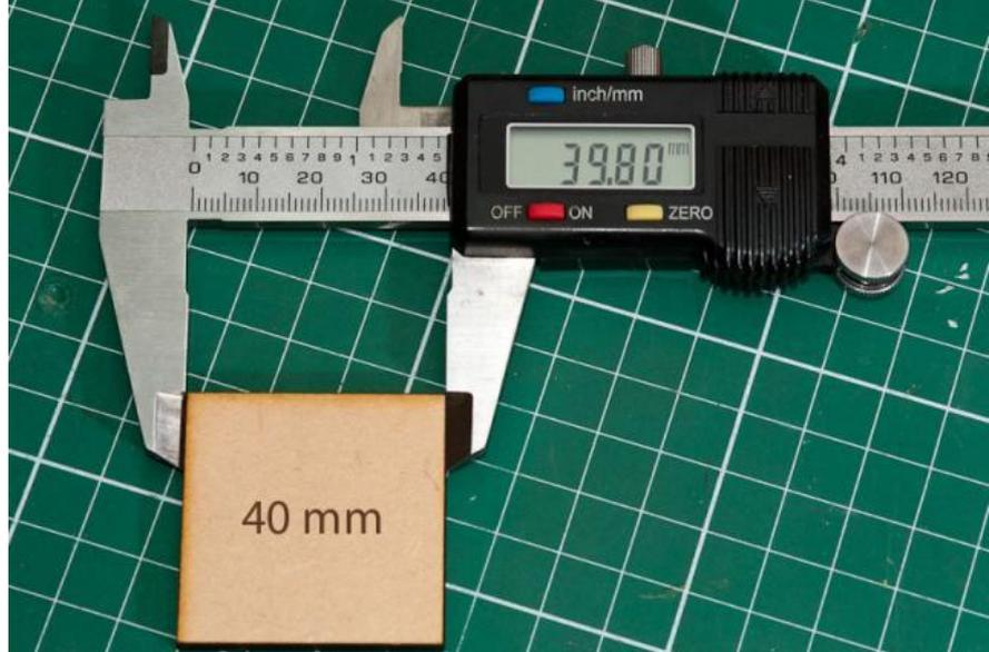
**Every cutting tool creates a cutting pathway, called a kerf. The width of the kerf of a laser cutter is typically 0.2mm, or the width of a human hair. We can incorporate this into our designs to get very accurate parts.**
