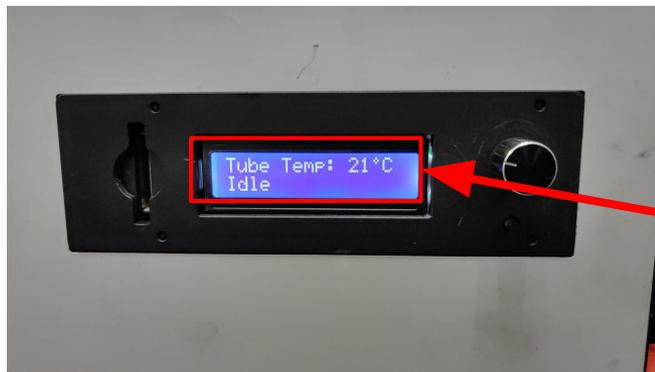
**Open the material loading tray when the display reads “Idle”. This is to ensure that the machine is done cutting/rastering. Check on the monitor and display to confirm the machine is done cutting before opening the tray.**
