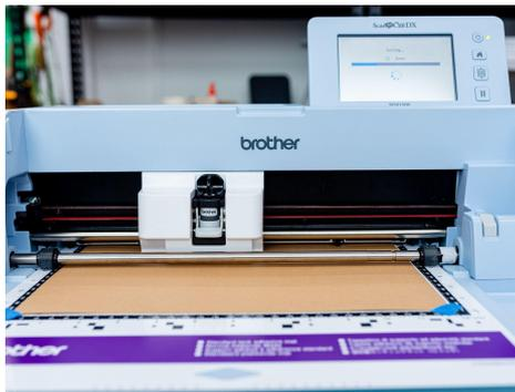
A bladed cutting head presses into cutting material, controlled by a computer.
