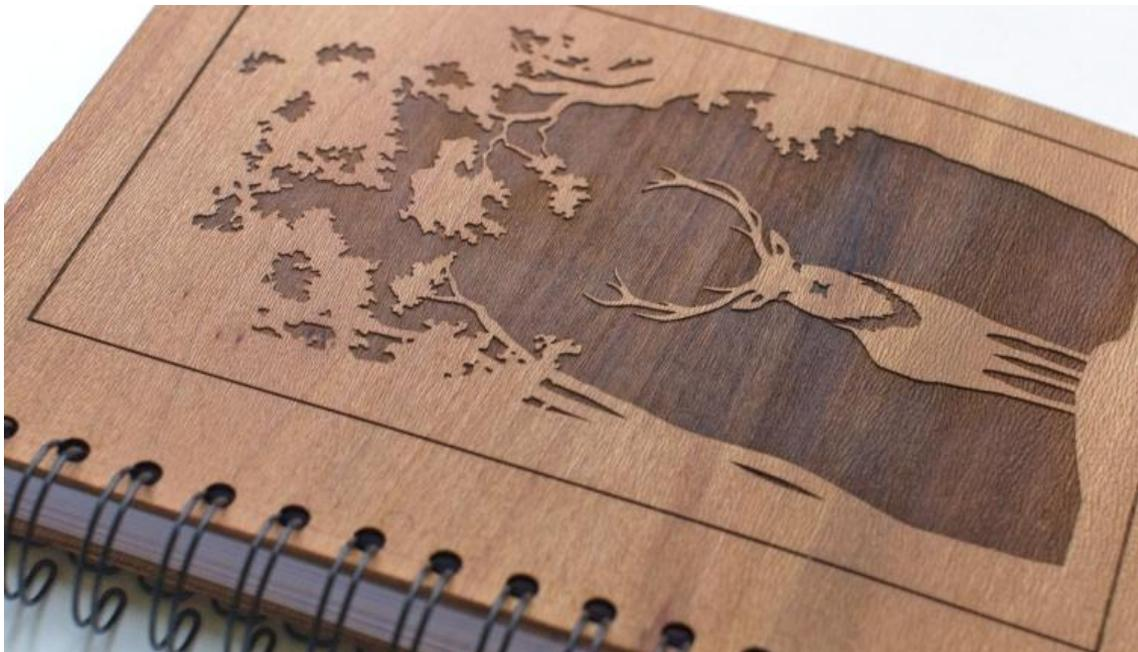
**Engraving changes an image into a feature where just the top layer is burned off. The thickness of the engraving depends on your speed and power settings.**
