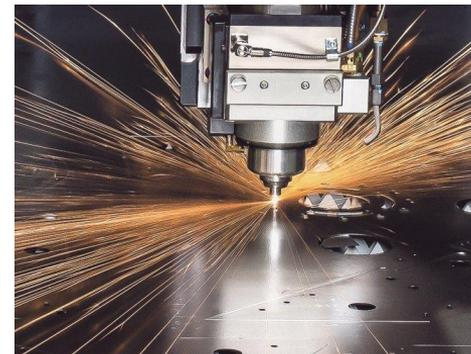
A laser beam fires into cutting material, controlled by a computer.
