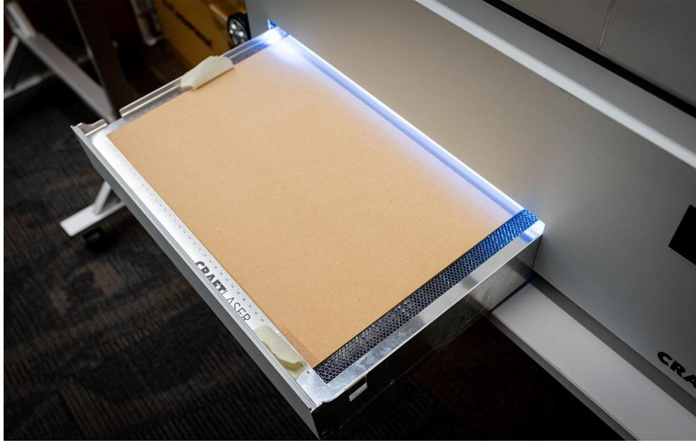
Medium-Density Fibreboard (MDF) is easy to use and is durable for laser cutting projects. It is made by combining wood fibres together with a binding agent, then is pressurized. The boards can be different thicknesses and colours, and can be used to make furniture, panelling, and DIY projects.
