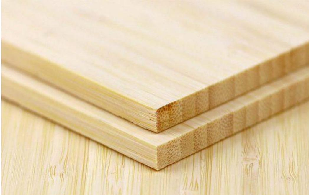
Bamboo plywood is an engineering wood, like MDF, but consists of strips of bamboo wood that are pressed and bound together. Bamboo plywood looks like wood, but is significantly cheaper.
