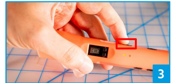
3 Select the appropriate temperature mode (H-PLA) by pressing the retract button [Big button beside indicator LEDs] until you see the letter H.
