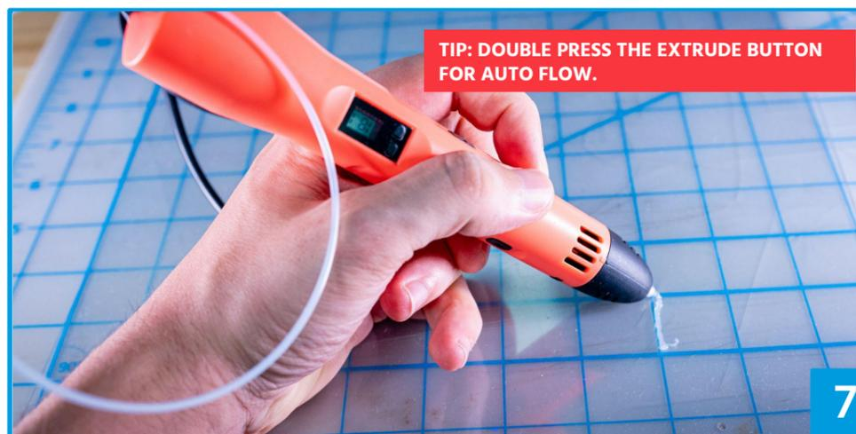
NOTE: While Operating 3D Pen, do not touch the nozzle as it is hot. Wait 20-25 seconds before the filament comes out. Press and hold the extrude button to draw, and let go of the extrude button to stop. Draw with the nozzle slowly, and press directly against a transparency sheet. The slower your nozzle travels and the closer it is to your transparency surface, the better your result will be.
